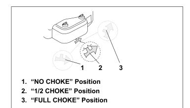
Figure 12. Engine Mounted Choke Lever
